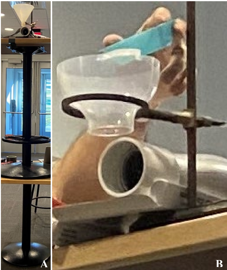
Figure 3. Experimental setup for the airborne time and dispersal distance of Cercis canadensis and Asclepias subulata . A. Overall setup. Note the narrower exit neck of the funnel used for C. canadensis seedpods. B. Closeup of setup used for A. subulata .
